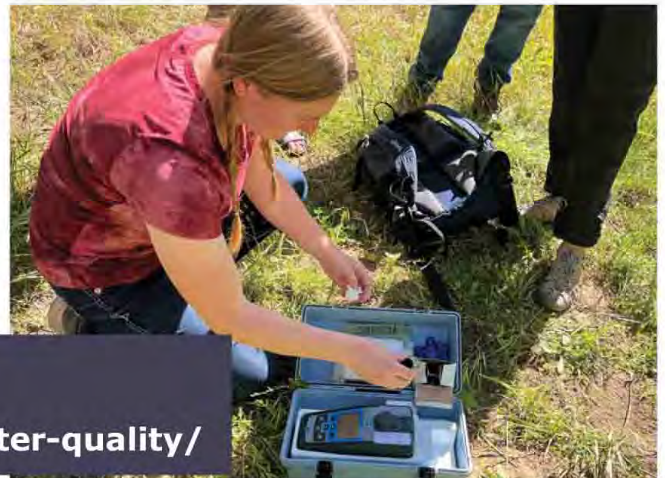
Yavapai Flood Control District staff prep the turbidimeter to check the clarity of the water using their stream sample
