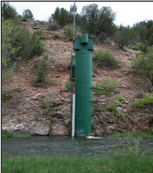
Figure 6.4. USGS Paulden Gage. Photograph of streamgage USGS 09503700 Verde River near Paulden. Courtesy of Gary Beverly.
